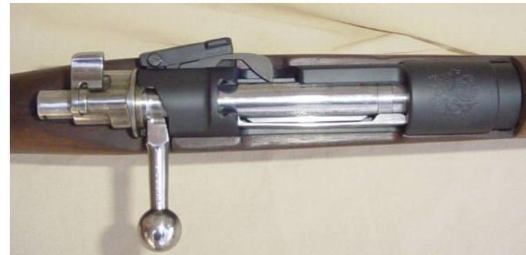
How the ejector should look when installed correctly
