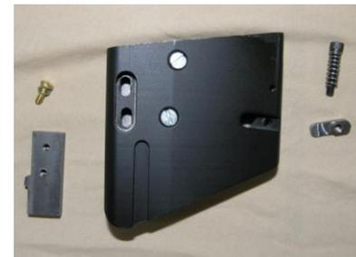
**Adapter: rear mag catch on the left (it is adjustable), main 1911 mag catch on the right.**
